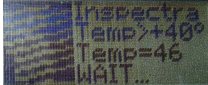
“Wait” message – Detector outside the authorized temperature range
